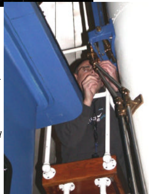
▶ Volunteer Telescope Operator Gerald McKeegan fixes a linkage problem on Chabot's 20" refractor, Rachel. A tapered pin fell out of a joint, rendering one of the telescope's locks inoperative. Gerald donated two bags of different-sized pins so future "pin problems" won't be quite so painful. (Photo by Don Saito)
